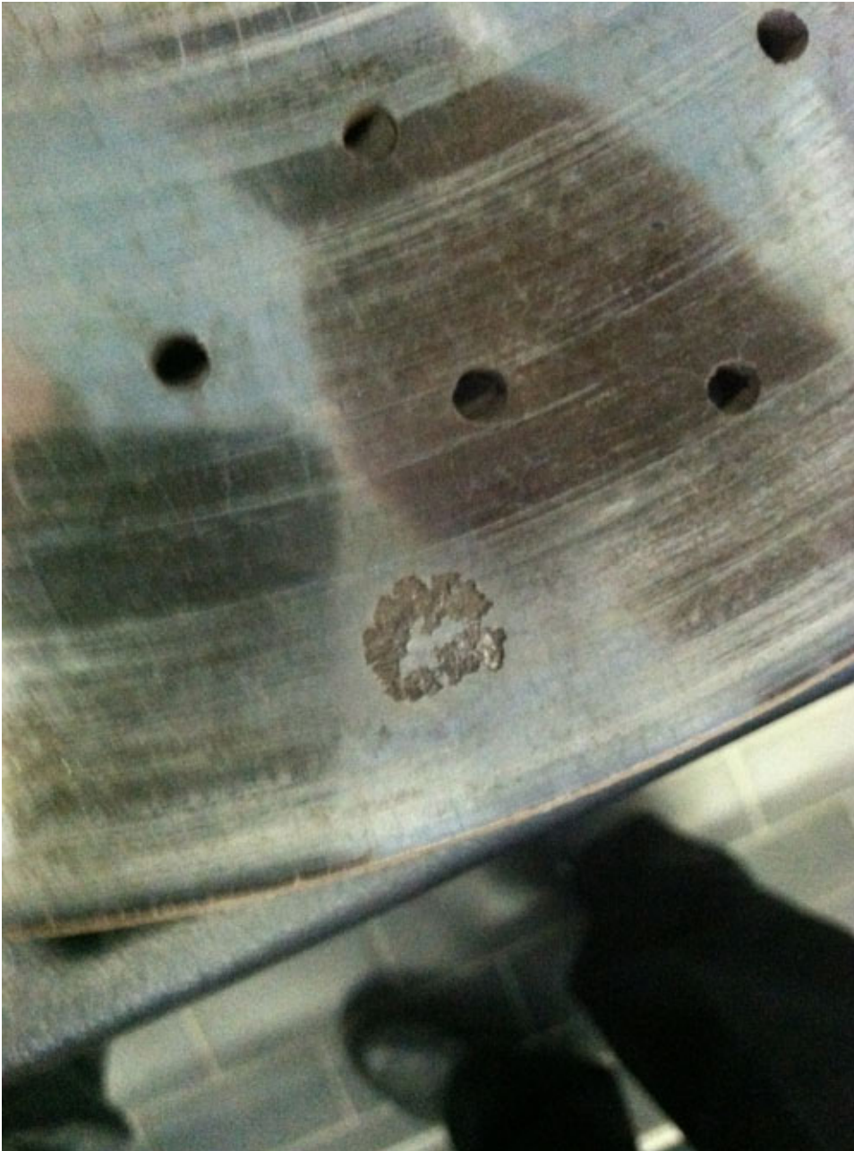
Disc must be replaced, total wear
