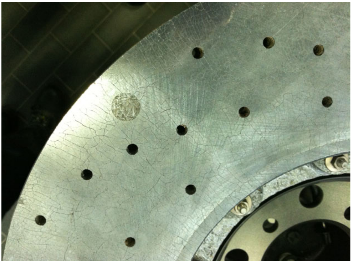
M Carbon ceramic brake, relaxed microstructure
