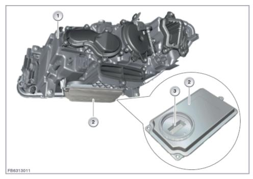
ItemExplanationItemExplanation1Right headlight, general view from<br/>rear2LED main headlight module on the<br/>right (LHMR)332-pin plug connection
