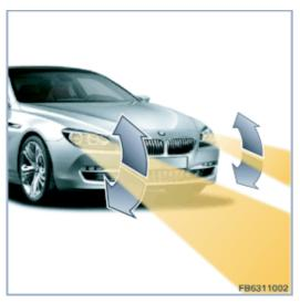
The adaptive headlight beam throw adjustment is employed when driving through dips and over crests. Depending on the request from the footwell module (FRM) or the Body Domain Controller (BDC), the headlight driver module controls the swivel module using the stepper motors and therefore controls the headlight beam throw of the headlight.
