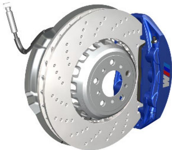
The front brakes are specific to the F10 M5. It uses a large ventilated M Compound brake discs combined with a six-piston fixed calipers. In comparison to the F10 550i, the diameter of the front brake disc @ 15.7 in is 1.02 in larger.
