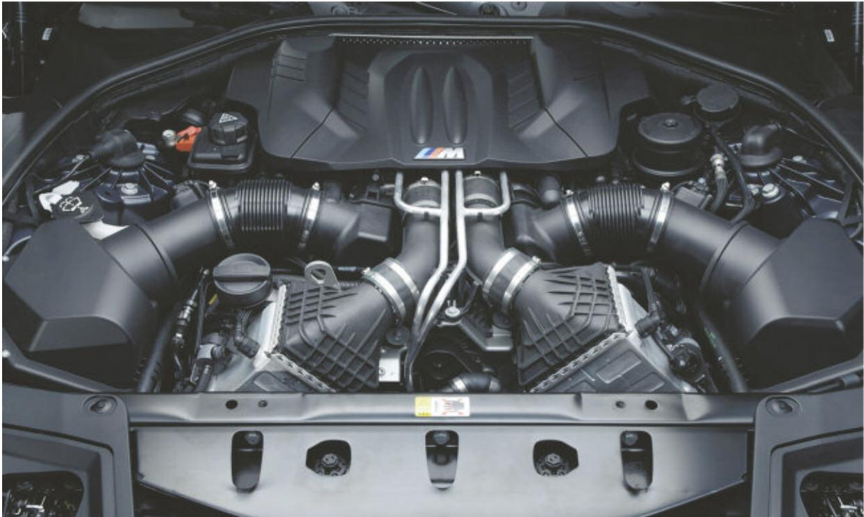
There is a new air duct for the center cooler module and for the side mounted M5 specific low temperature cooler. The lower engine compartment shielding is a single piece. (Standard F10: 3-piece).
