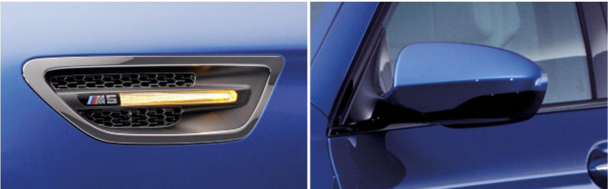
The familiar M gills with the integrated side directional lights are mounted on the front fenders.
