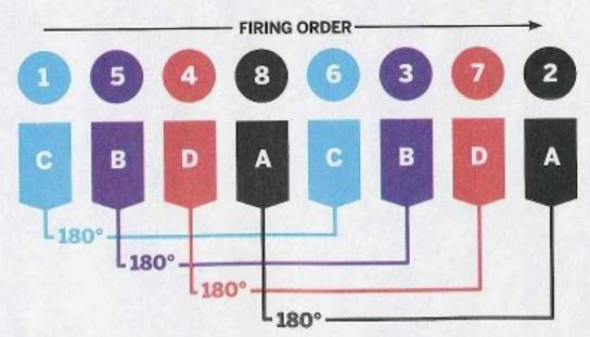
EVEN INTERVAL BETWEEN EXHAUST PULSES. Each turbo receives an exhaust pulse every 90° of crankshaft rotation, alternating evenly between its two inlets.
