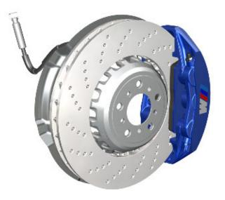
The front brakes are specific to the F10 M5. It uses a large ventilated M Compound brake discs combined with a six-piston fixed calipers. In comparison to the F10 550i, the diameter of the front brake disc @ 15.7 in is 1.02 in larger.
