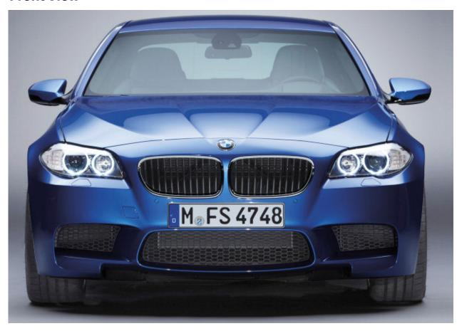
The bumper has been designed specifically for the M5. The lower area of the bumper reduces lift at the front axle. The PDC sensors are painted in the vehicle color. No fog lights are installed due to the large air inlets.
