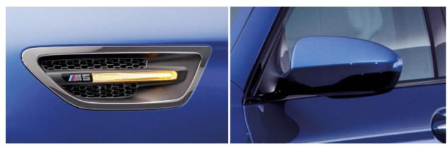
The familiar M gills with the integrated side directional lights are mounted on the front fenders.
