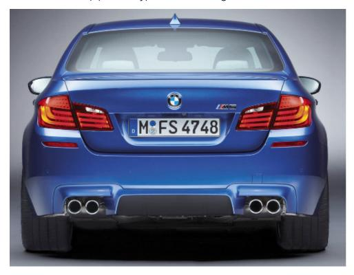
The rear diffuser in the rear bumper between the tail pipes and the rear spoiler on the trunk lid reduce the rear axle lift. The trunk also incorporates the rear view camera as standard and the power tailgate is optional.
