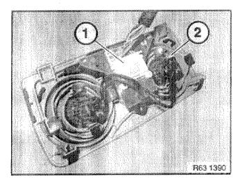
Unfasten plug connection (1) and disconnect. Remove interior roof light (2).
