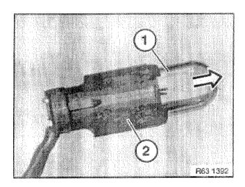
Pull bulb (1) out of bulb holder (2) in direction of arrow.
