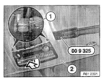
Unlock retaining lugs (1) with suitable tool while carefully lifting out with special tool <u>00 9 325</u>.
