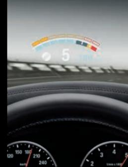
The BMW Head-Up Display with M-specific display projects all relevant driving data and, if requested, Speed Limit Info directly onto the windshield.
