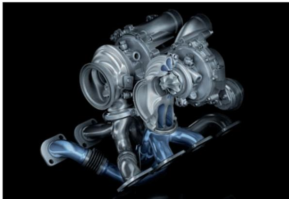
**TwinScroll turbocharger with a cross-bank exhaust manifold:** the exhaust flows from each of two cylinder pairs with a 360° firing interval are combined and routed along separate channels before reaching the turbine wheels of the turbochargers. This guarantees that gas flow is not compromised. It's a highly efficient charging concept that leads to optimum energy transfer – and, therefore, extremely spontaneous responsiveness.
