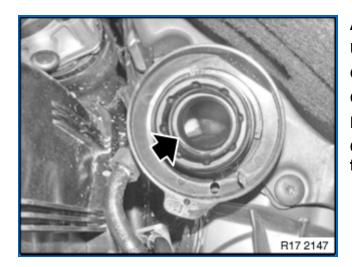
Adding coolant: Use <u>only recommended coolant</u>. Observe <u>mixture ratio</u>. Observe <u>filling capacities</u>. Fill and vent <u>cooling system</u>. Observe bleeding instructions without fail.
