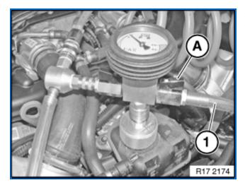
valve (A) again. The filling hose (1) is vented in this way.
