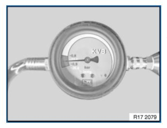
meter falls, this indicates a leak in the cooling system.
