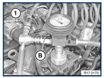
Shutoff valve (B) remains open. Generate vacuum in cooling cycle for approx. 1 minute. The end vacuum is reached at a vacuum of -0.7 to -0.95 bar. Green scale on the vacuum meter.
