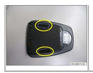
picture. Reassemble the modified speaker cover to the speaker. Quality check the repair by road testing the vehicle and confirm the noise has been eliminated.
