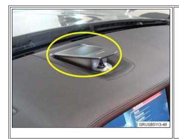
1. Use ISTA Repair Instruction 65 13 052 to remove the loudspeaker cover from the speaker.
